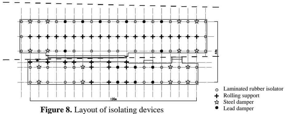
Figure 8. Layout of isolating devices
