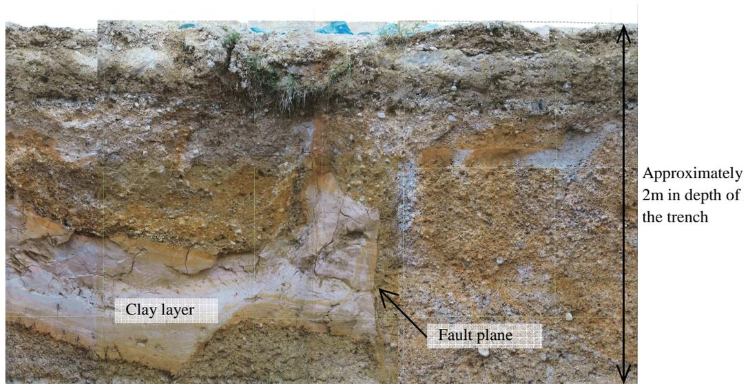
**Figure 6.** Orthogonal cross section of the active fault confirmed in the cross section of the trenched fault
