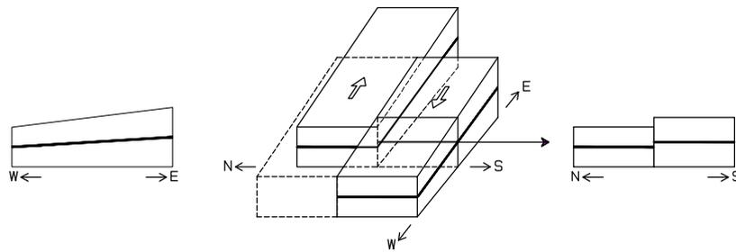
**Figure 7.** Explanatory diagram of a sloping fault that becomes discontinuous by horizontal placement attributable to a strike-slip fault
