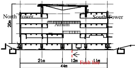
**Figure 4.** Cross section of the building
