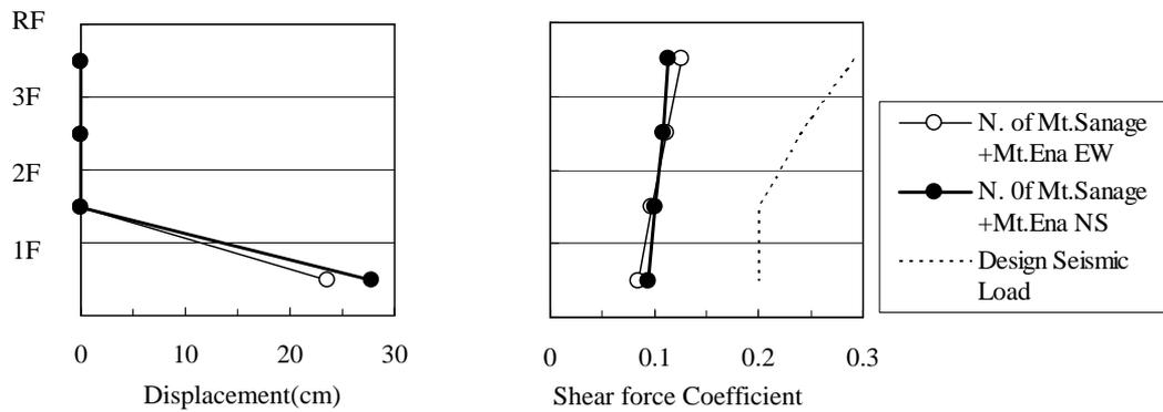
Figure 9. Results of responses analysis of the building to level 3B earthquakes
