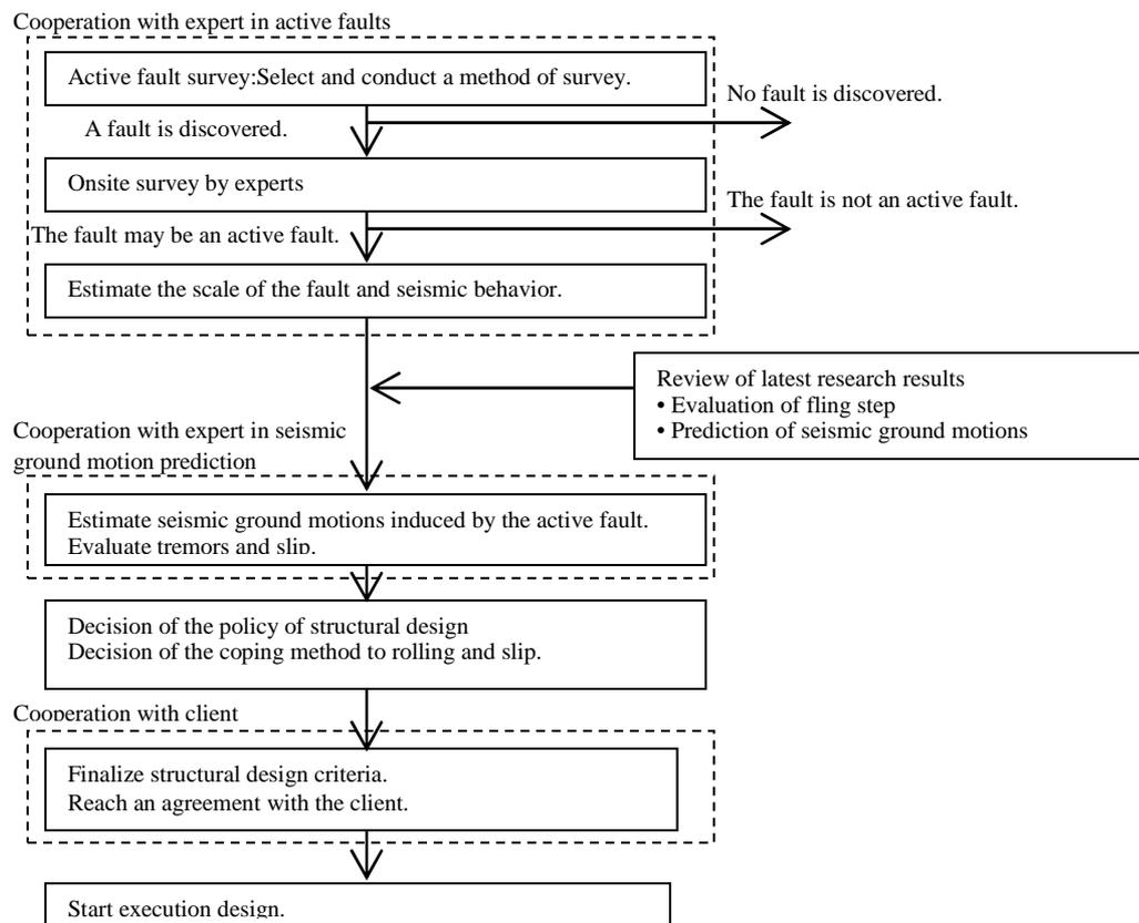
**Figure 11.** Flow of fault survey in architectural design
