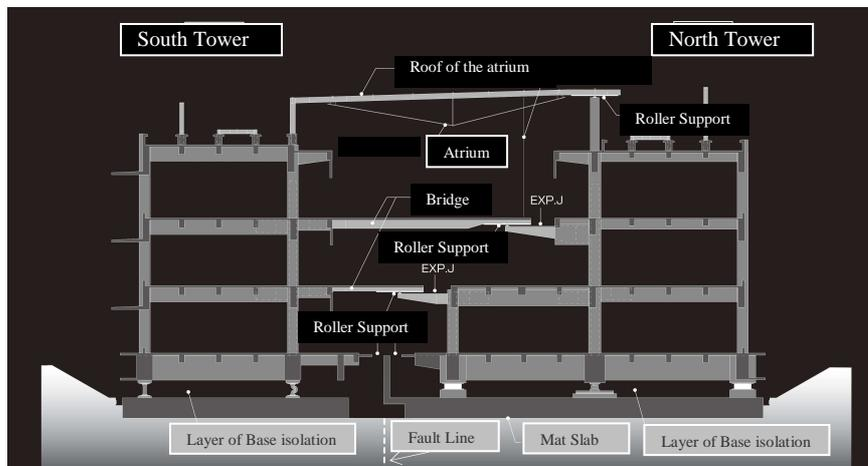
Figure 10. Conceptual diagram of structural design
