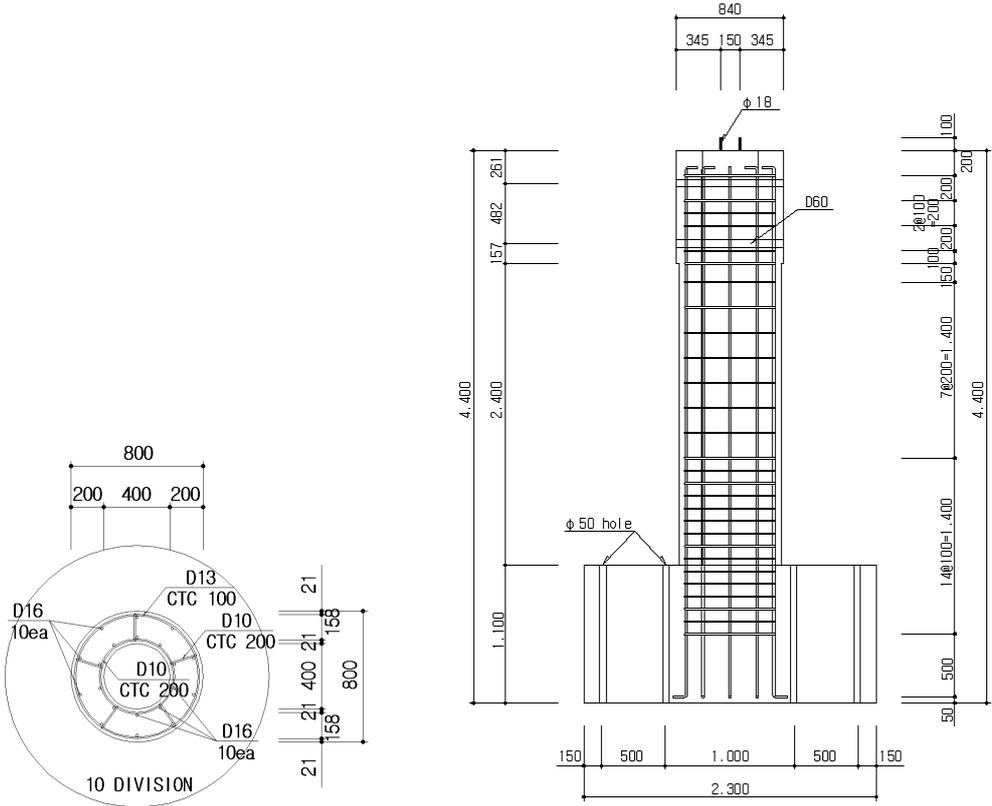
**Figure 1.** Sample of test specimens HC-O-100 (Unit: mm)
