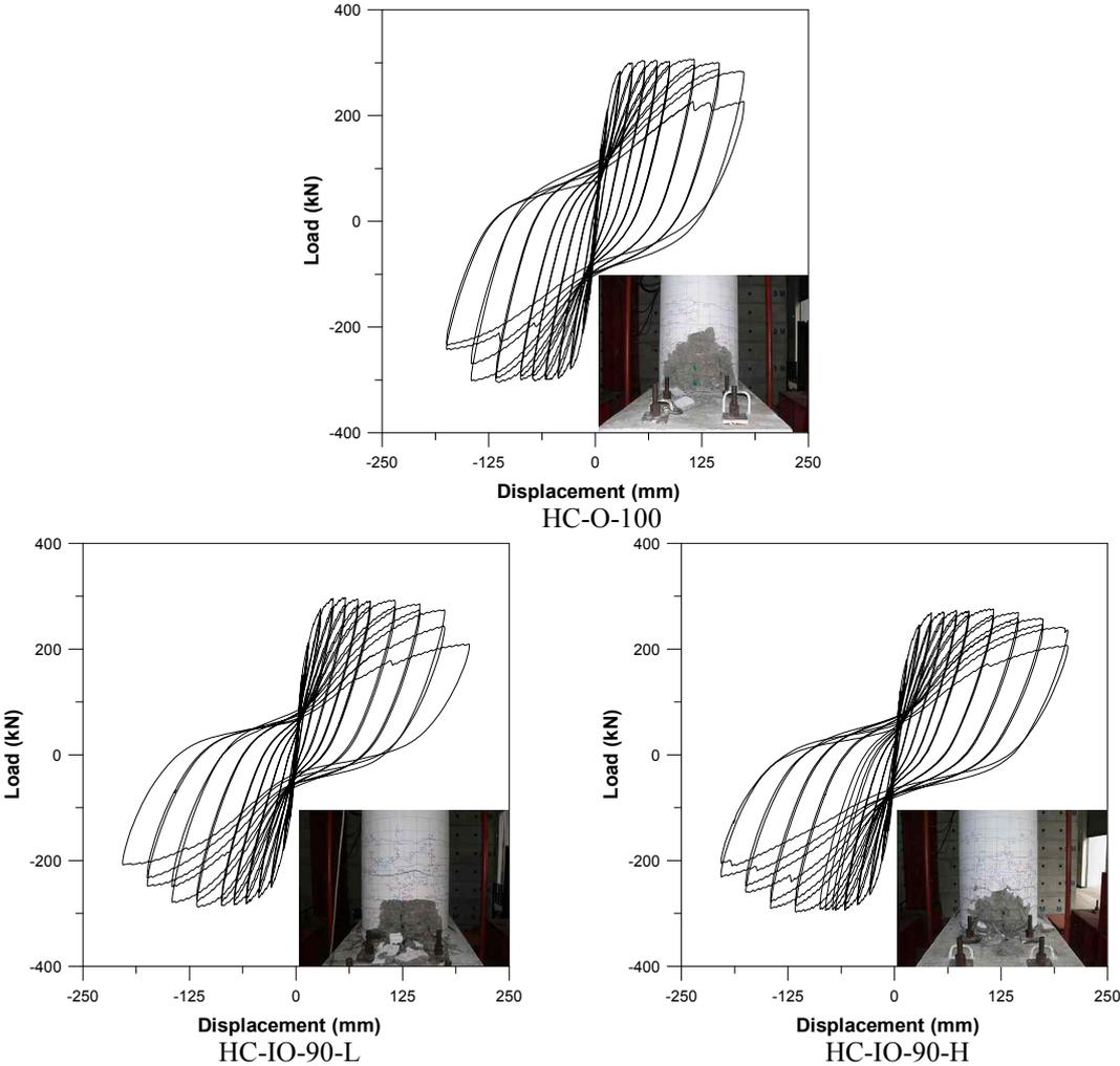
Figure 3. Load-displacement relationship for specimens
