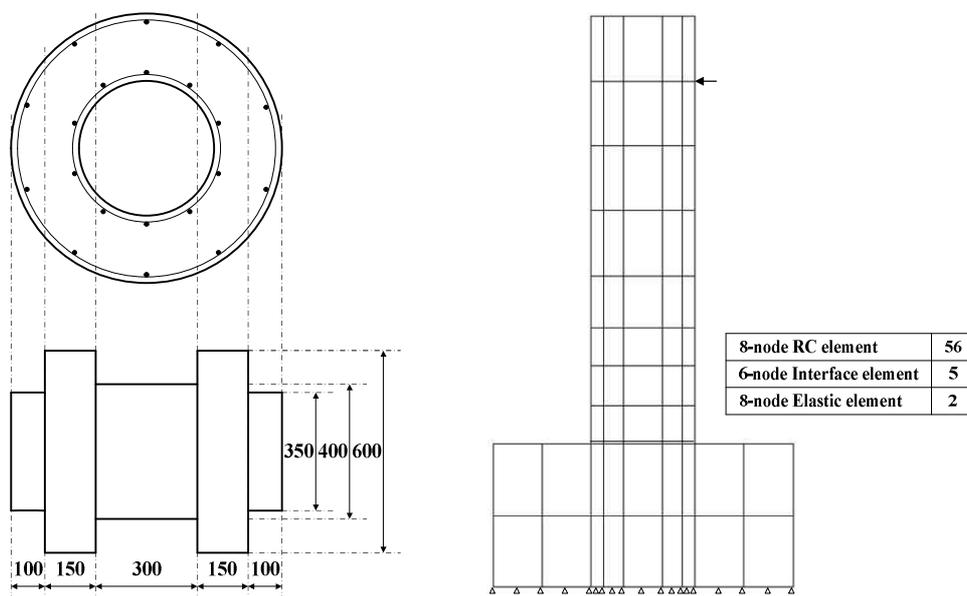
Figure 4. Finite element model for specimen
