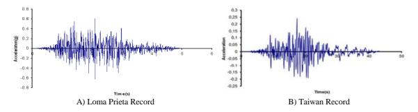
Figure 4: Two Near-Fault Earthquakes
