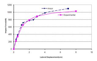
Figure 11. Comparison of results obtained with ANSYS and with the experimental analysis
