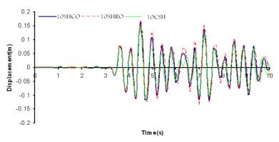
Figure 6: Time history of displacements under Taiwan earthquake
