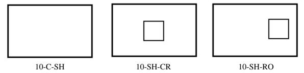
Figure 3: Three different shapes of opening
