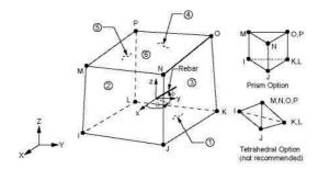
Figure 9. Solid element (SOLID 65) in ANSYS
