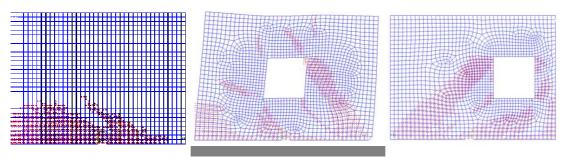
Figure 12. Crack patterns of the three analysed panel models
