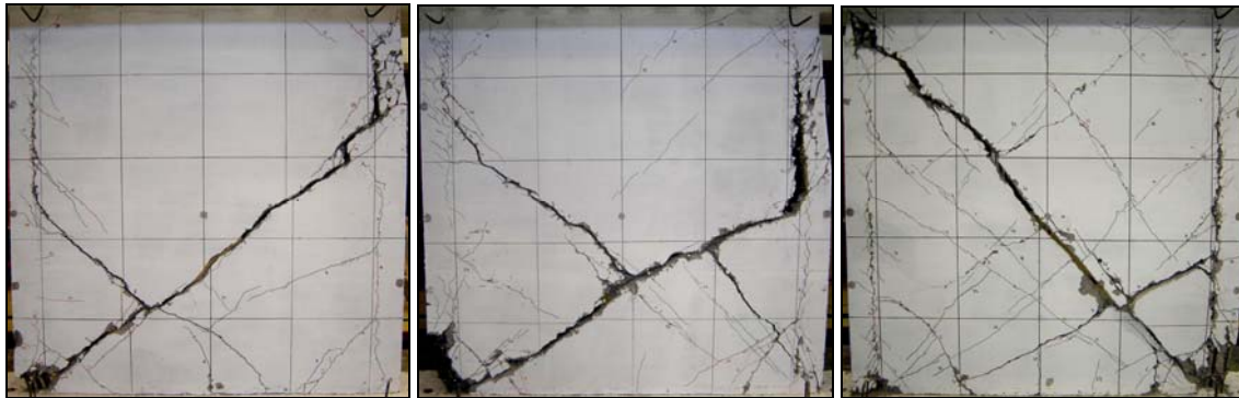
Figure 7. Final crack patterns of walls with fiber type 2F: (a) MC2F75, (b) MC2F100, (c) MC2F125.
