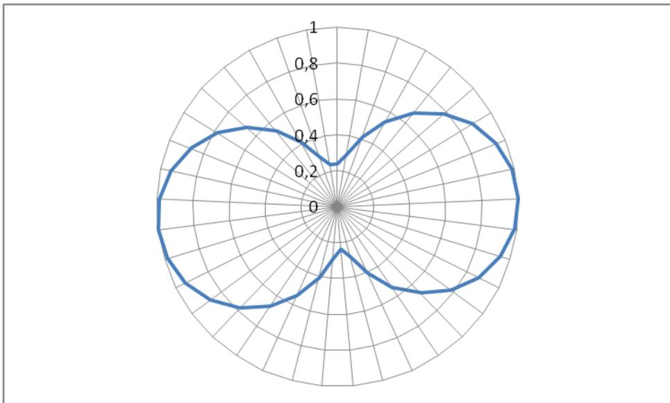
**Figure 8. Booth curve, bean-shaped, for the deflections ellipse of the figure 6.**
