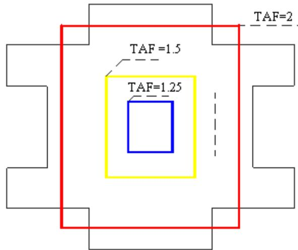
**Figure 5: Central torsional kernels referred to the Torsional Amplification Factor (TAF) =2, TAF = 1.5 y TAF =1.25)**
