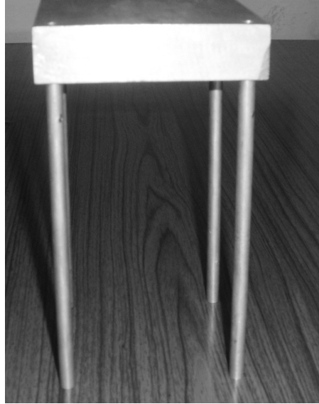
Figure 1. Model pile group with L/d = 15 .
