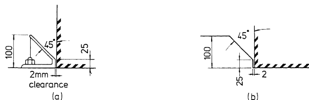
Fig. 7 Methods of restraining lead-rubber bearing, (a) on flat foundation and (b) in recess in foundation.
