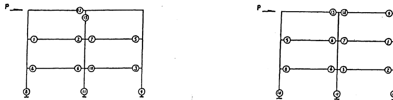
a) Test Results ( P_y = 163 \text{ kN} , \Delta_y = 2.89 \text{ cm} ) b) Analysis Results ( P_y = 151 \text{ kN} , \Delta_y = 2.64 \text{ cm} )
