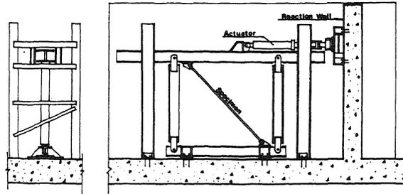
Fig. 1 Testing Frame and Reaction Wall
