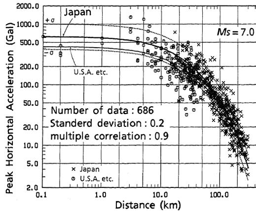
Fig. 8 Comparison of new attenuation relationships for Japan and for U.S.A. etc. with data points normalized to  $M_s 7.0$
