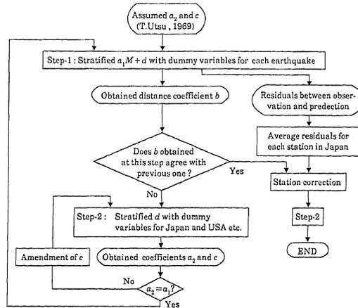
Fig. 7 Procedure of two-step stratified regression analyses
