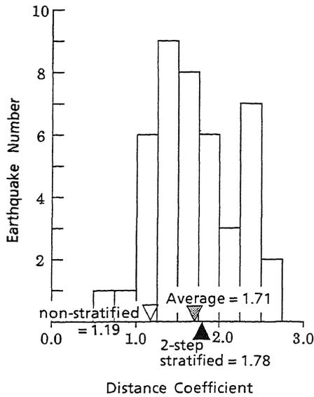
Fig. 4 Histogram of distance coefficients of individual earthquakes. The coefficients by non-stratified and two-step stratified regression analyses are indicated by triangles.
