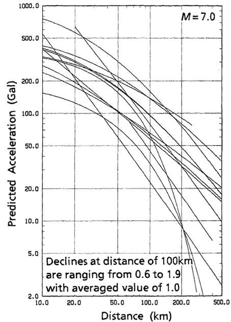
Fig.1 Attenuation relations for PGA proposed within the last 10 years (1977~1987) in Japan
