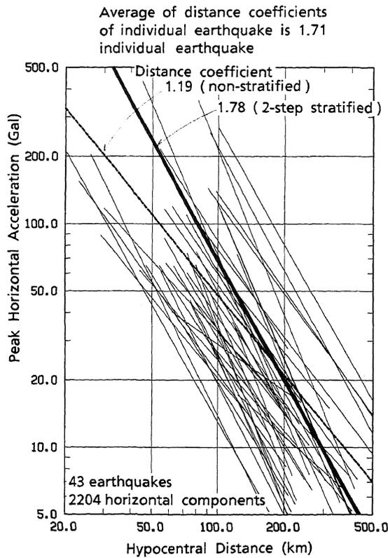
Fig.2 Comparison of attenuation relationships by non-stratified and two-step stratified regression analyses, and those for individual earthquakes
