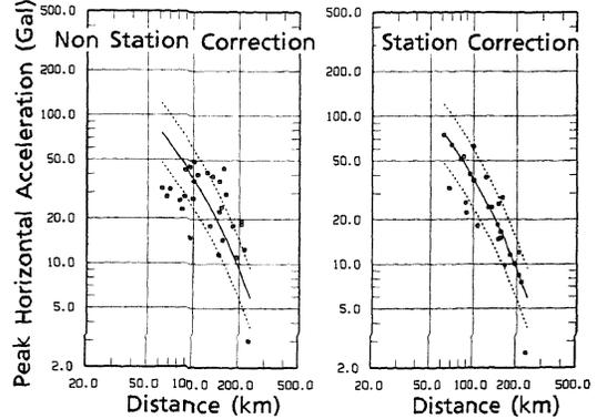
Fig.11 Comparisons between the observed and predicted PGA
