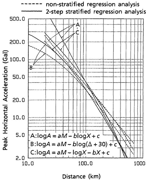
Fig. 5 Comparison of attenuation relationships by non-stratified and two-step stratified regression analyses for typical models in Japan
