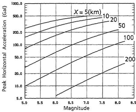
Fig.9 Predicted PGA by the new attenuation relationships as a function of distance and magnitude
