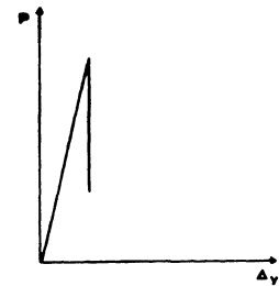
Fig.12: Load P versus displacement \Delta_y (typical plot).
