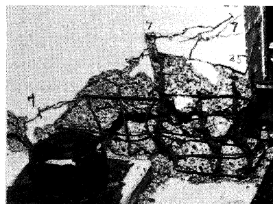
Fig. 11 Shear Wall--Frame Base Crushing
