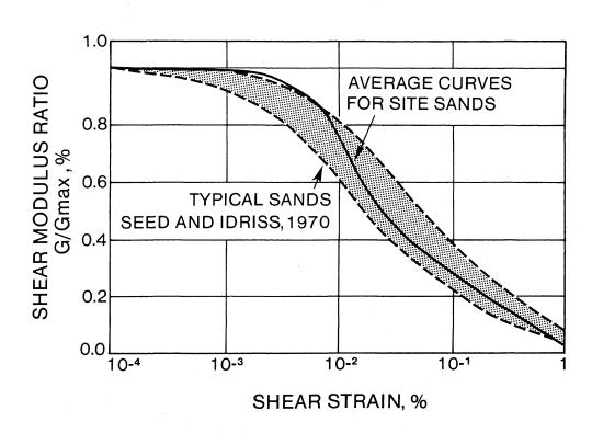
FIG. 2. - VARIATION OF  $G/G_{\mbox{\scriptsize MAX}}$  WITH SHEAR STRAIN
