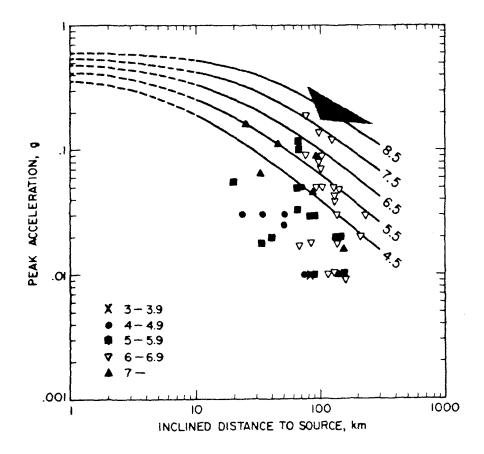
Figure 2. Comparison of Alaska peak horizontal accelerations with B-type attenuation relations proposed by Woodward-Clyde (Ref. 7) for Benioff-zone earthquakes. Curves are for stiff sites and represent the median. For other details compare legend of Figure 1. The stippled field represents Japanese peak acceleration data for the  $M_W \approx 8.2~(M_B = 7.9)$  Tokachi-Oki earthquake (Ref. 5) discussed in the text.
