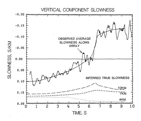
Figure 2. Jagged line is observed slowness of vertical ground motions along the array during the earthquake, and smooth line is fit visually through the observations. Dashed and dotted lines are true slownesses inferred from the smoothed observations, based on indicated source depths. Negative slownesses indicate energy travelling in a southerly direction, positive indicate northerly propagation.
