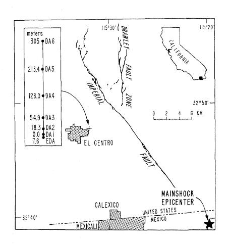
Figure 1. Location and layout of the array elements, and surface rupture associated with the earthquake. EDA was an analog SMA-1 accelerograph.
