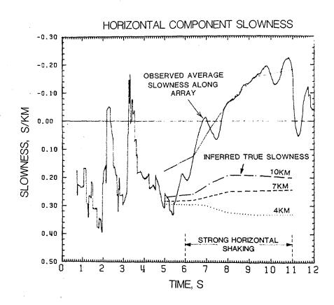
Figure 3. Observed and true slowness of horizontal ground motions. See Figure 2 for details.
