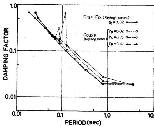
Fig.10 Coupled Damping of Rayleigh Type
