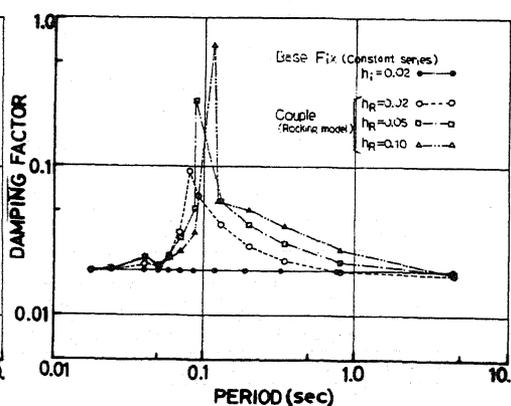
Fig.11 Coupled Damping of Constant Type
