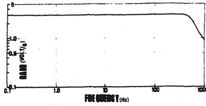
Fig.2 Gain Characteristics
