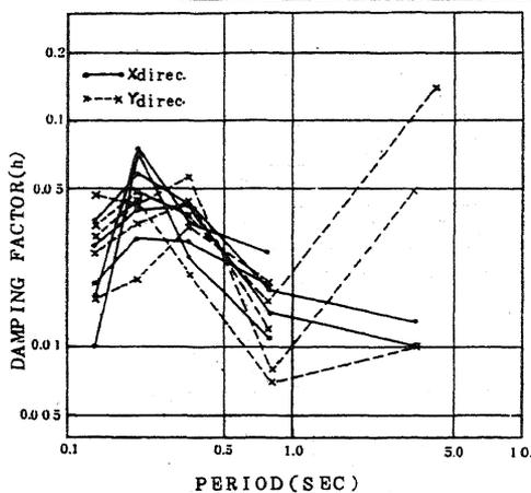
Fig.9 Damping Factor and Period
