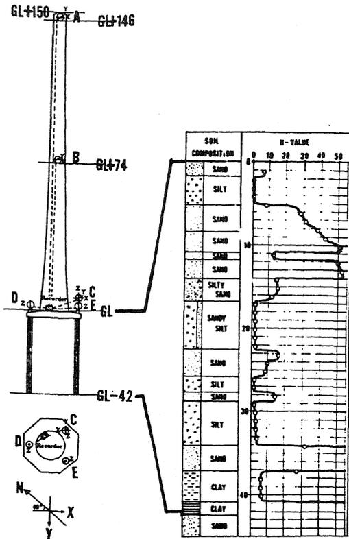
Fig.1 Location of Seismograph
