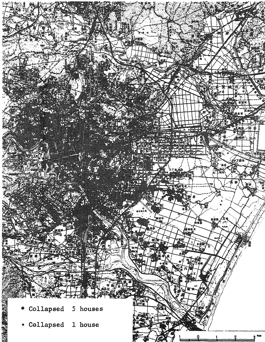
Fig. 1 Distribution of collapsed houses in Sendai City
