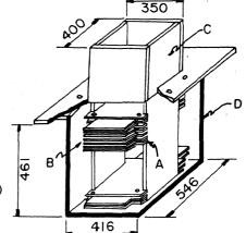
By adjusting gap and area of the plates, the longitudinal horizontal force can be distributed uniformly even to the piers with various stiffness. Such a stopper is easily changeable to a type of stopper which is movable to any direction to work as an energy absorption divice.
