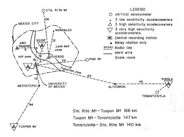
Fig 1. Layout of SISMEX network
