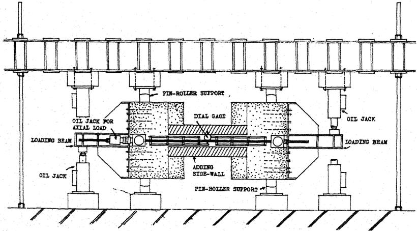
Fig.6 TEST FACILITY FOR SERIES-CW
