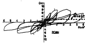
Fig. 9 Q - δ CURVE OF SERIES-PCW, PCWH
