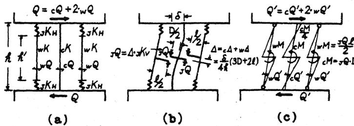
Fig. 15 IDEALIZED LOAD TRANSFER MODEL OF SERIES-CW, TYPE PA
