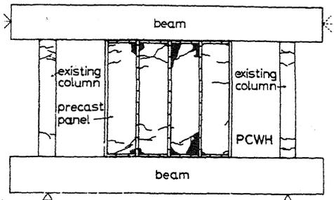
Fig. 12 CRACK PATTERN OF PCWH, SERIES-PCW
