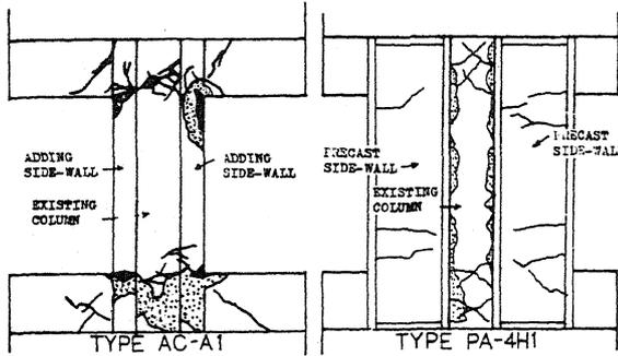
Fig. 10 CRACK PATTERN
