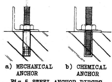
Fig.5 STEEL ANCHOR-PIECES
