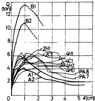
Fig. 13 ENVELOPES OF Q - δ CURVES, SERIES-CW
