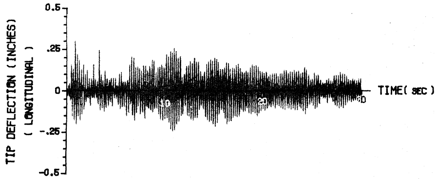
Fig. 7. Vertical tip deflection vs. time curve for outer shell.
