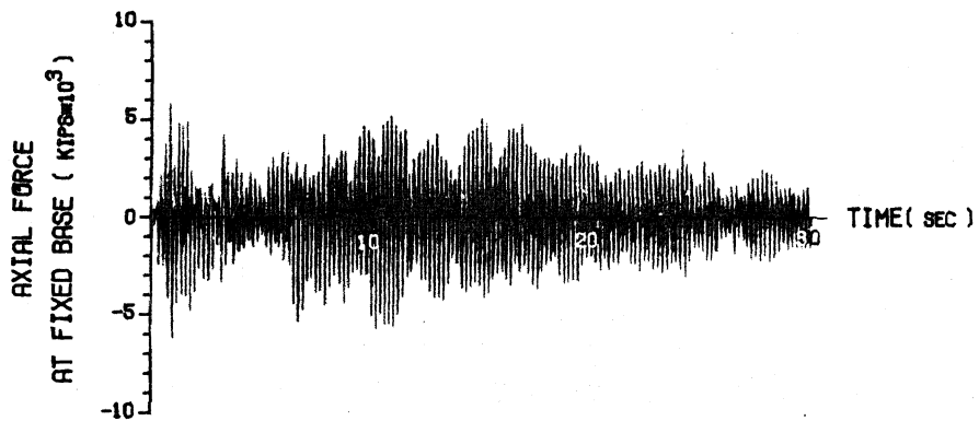
Fig. 8. Axial force at base vs. time curve for outer shell.
