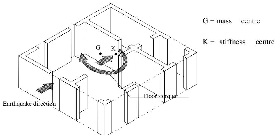
**Figure 3: Distribution of the seismic forces with the rigid floors option**
