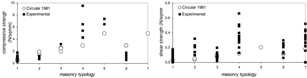
**Figure 4: Experimental vs. suggested values of ultimate stresses for various masonry typologies**
