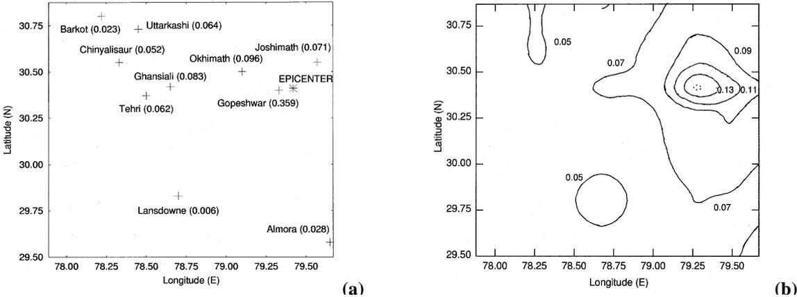
**Figure 2. Location of strong motion stations and contours of PGA**
