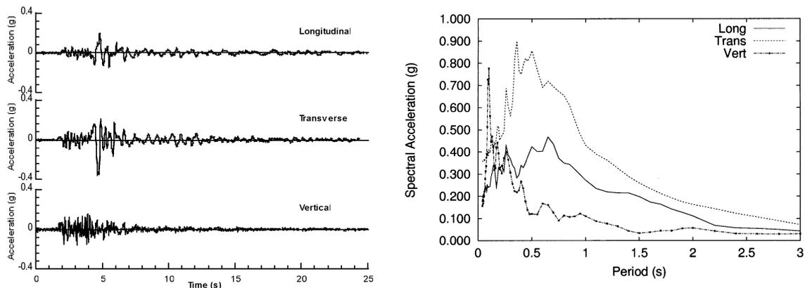
Figure 3. Recorded time histories at Gopeshwar and their spectral acceleration plots (5% damping)
