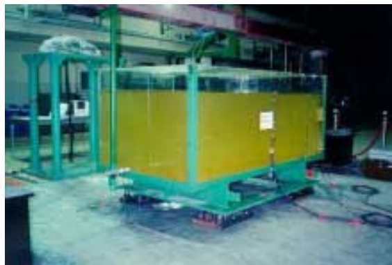
Figure 2. Shaking Table Test of Base Isolated Liquid Storage Structure
