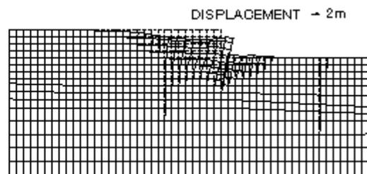
**Figure 12: Residual deformation (major section)**
