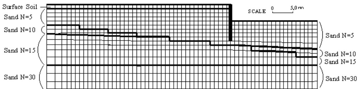
**Figure 9: Finite element mesh divisions of major section.**
