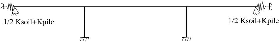
**Figure 2: Abutment stiffness for dynamic analysis**
