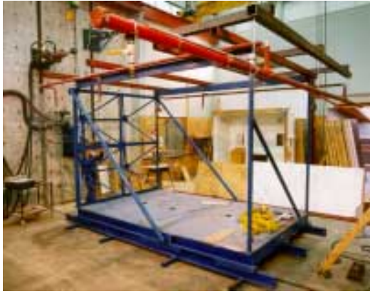
Figure 4 Sprinkler system on shake table
