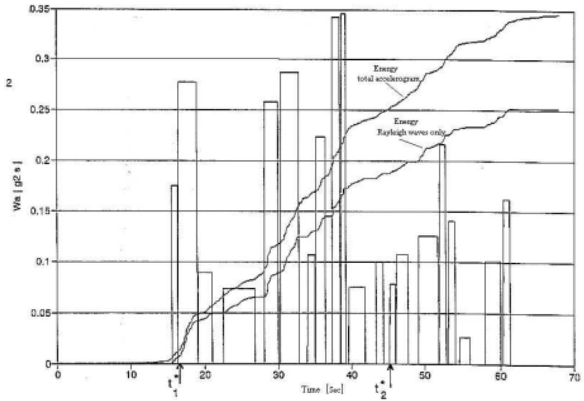
Fig. 2. Rayleigh Wave Effect on the Energy Function of the Accelerogram. Viña del Mar S20W.
