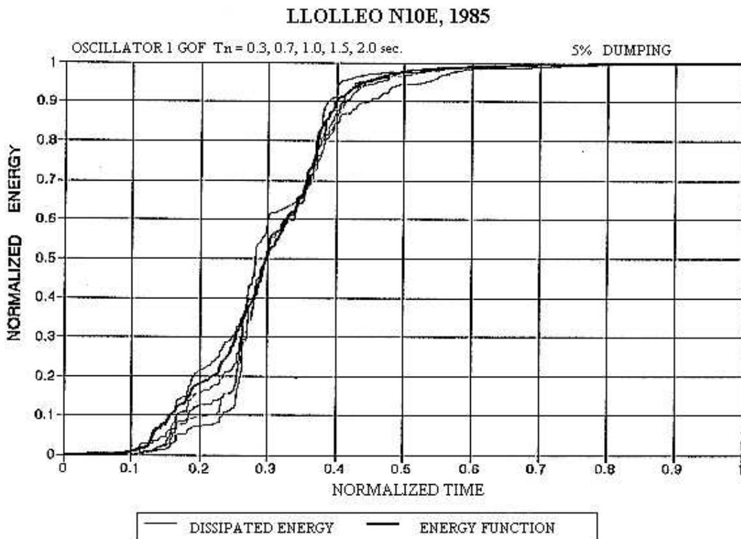
**Fig. 1. Comparison Between Dissipated Energy and Accelerogram Demand Energy Function for Kobe JMA NS. 1995 and Lollole N10°E.1985**
