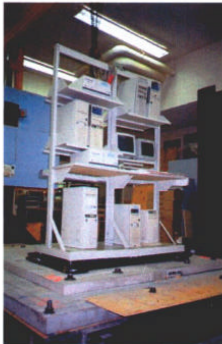
Figure 5 : Research of CFRP on Shear Walls and Shake Table Testing for Non-Structural Components
