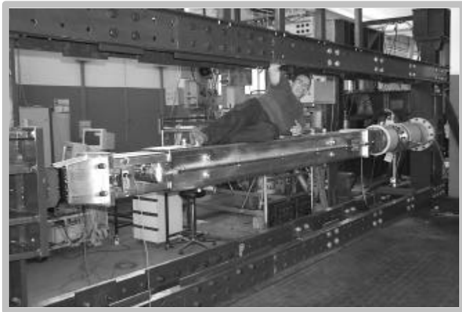
Figure 8. Full-scale isolator device ready to be tested.
