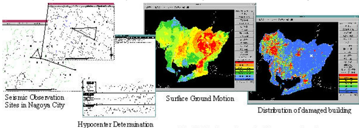
Fig. 8 Early earthquake damage estimation system
