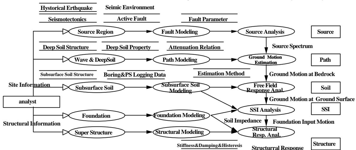
Fig. 3 Data flow in earthquake response analysis
