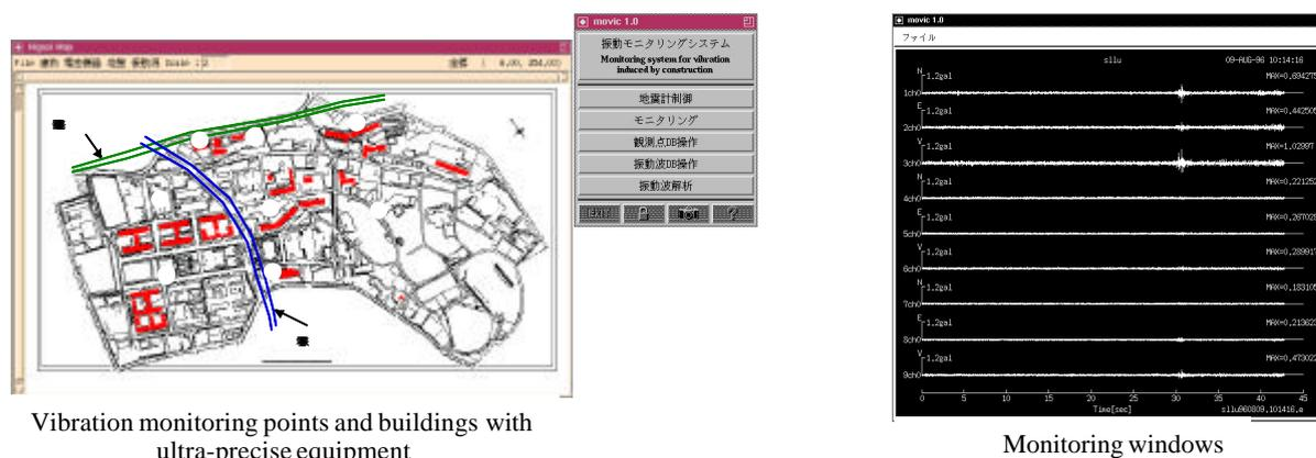
Fig. 9 Environment vibration alarm system
