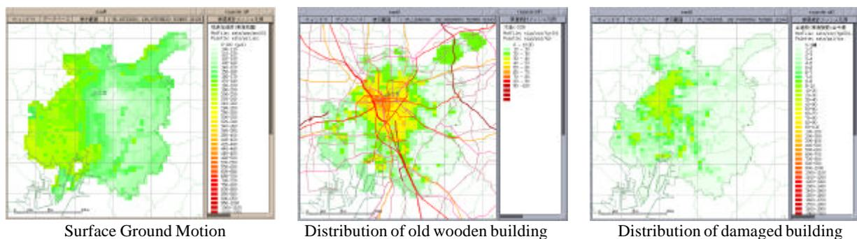
Fig. 7 GIS for earthquake damage estimation
