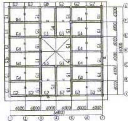
Fig.27 Typical floor plan
