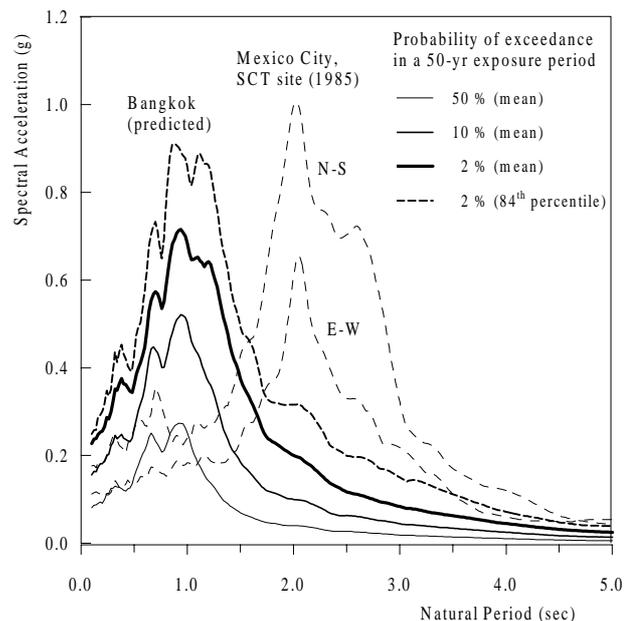
**Figure 5: Comparison between the elastic response spectra of predicted ground motions and the spectra of the damaging ground motions in Mexico City**
