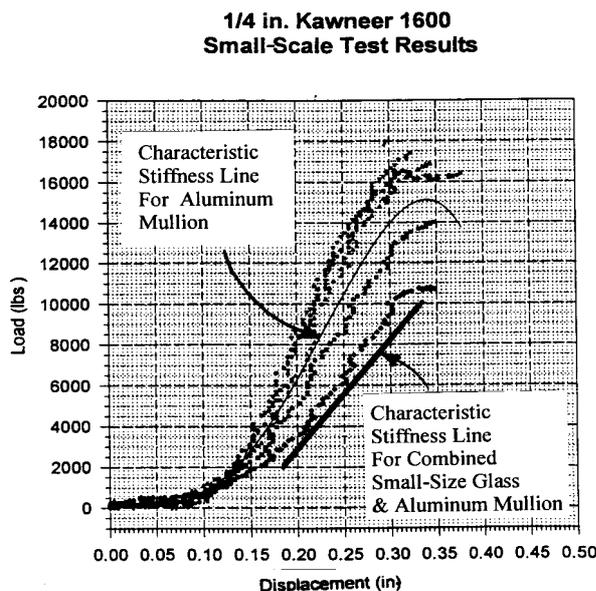
**Figure 4: Load-deformation data for Kawneer 1600™ shear block aluminum frame test.**
