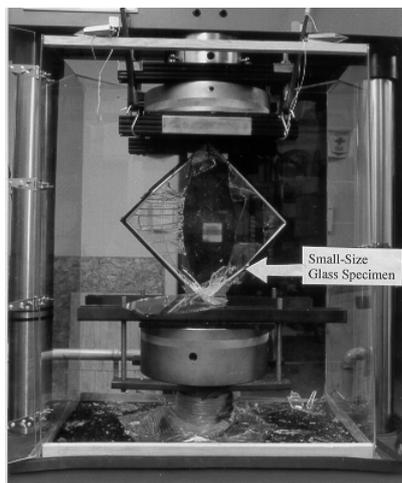
**Figure 1: Small-size glass test apparatus and typical small-size glass specimen. (Note: Specimen under test is a two pane insulating glass unit.)**
