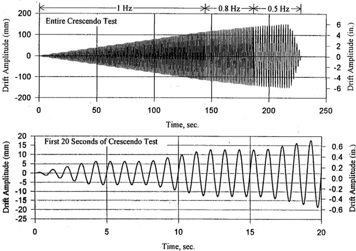
**Figure 6: A typical drift time history for performing dynamic racking crescendo tests.**
