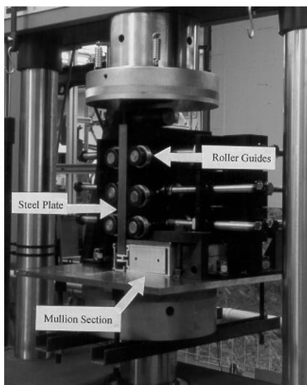
**Figure 3: Aluminum frame test apparatus.**
