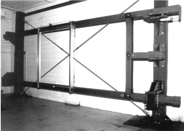
**Figure 5: Facility used for dynamic racking tests of full-size curtain wall panels.**
