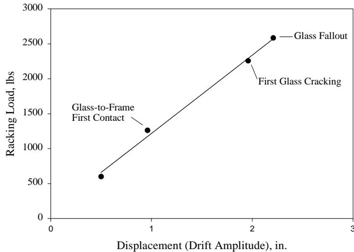
**Figure 7: Average load-displacement relation from full-size tests on sections of curtain wall glazed with 6 mm (1/4 in.) annealed monolithic glass and Kawneer 1600™ shear block aluminum frames.**
