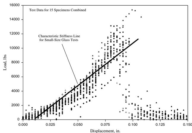
**Figure 2: Small-size glass load-deformation data for 1/4 in. annealed monolithic glass.**
