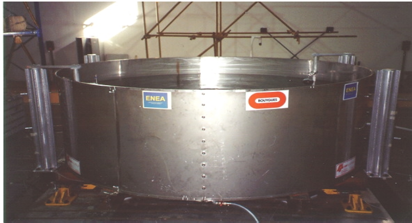
Figure 1: The LNG storage tank mock-up on the shaking table.
