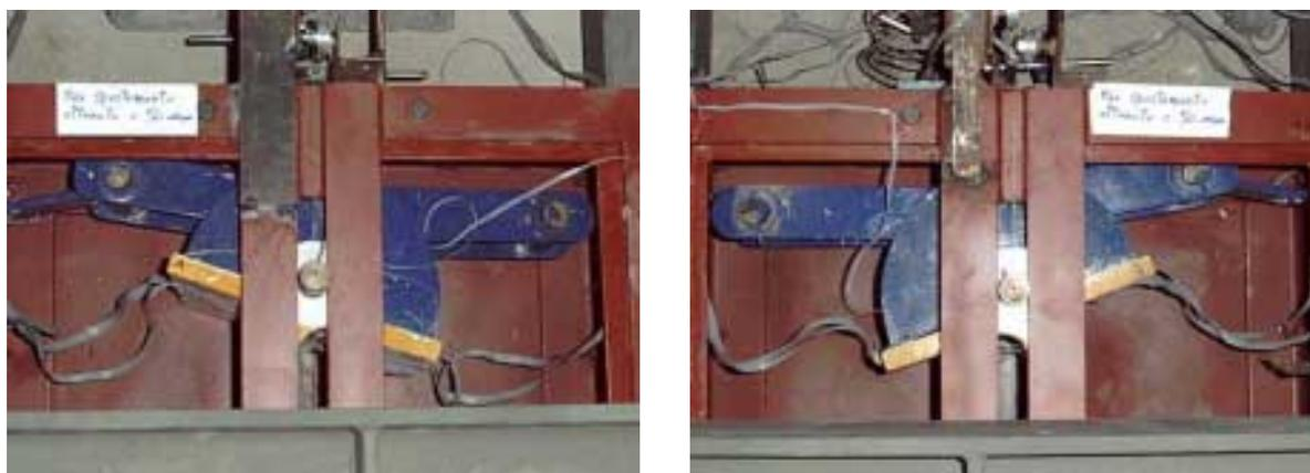
**Fig 10: A step of the experimental test: deformed elements (imposed displacement  $\pm 50$  mm)**
