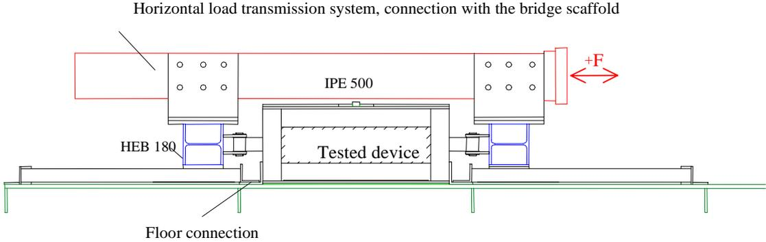
**Fig 6: Front view of the testing equipment**
