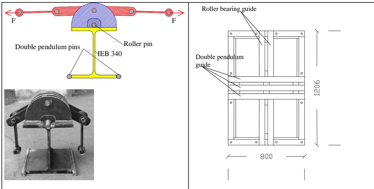
Fig 2: Single dissipating element-front view
