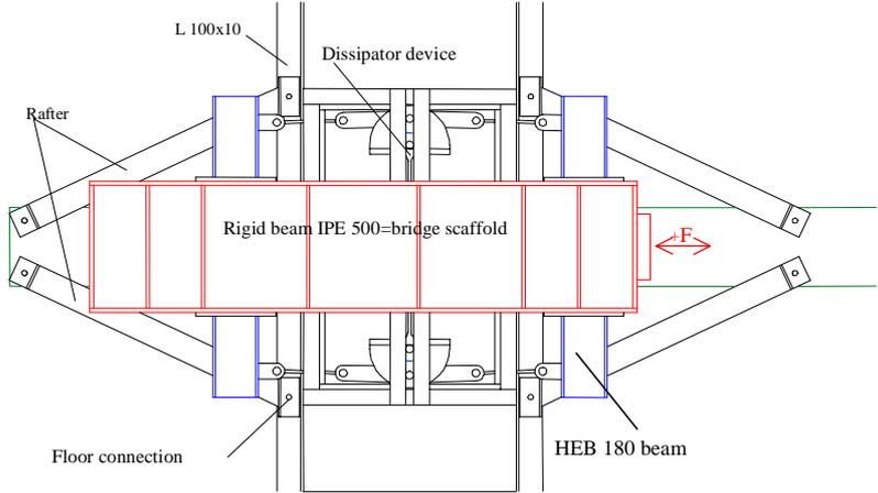
**Fig 5: Plan view of the testing equipment**
