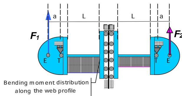
**Fig 1: Static scheme of the prototype**
