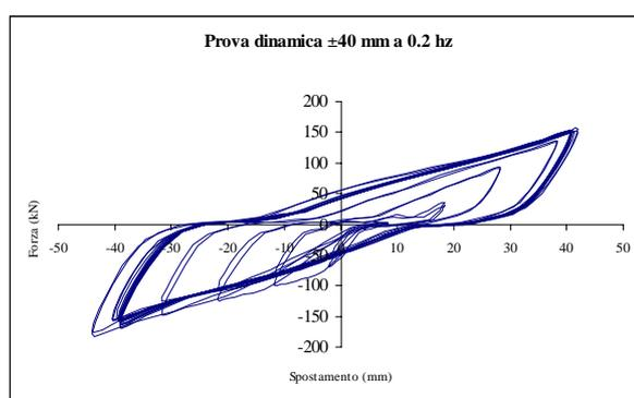
**Fig 9: Hysteresis loops obtained from the dynamic test**
