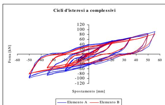
**Fig 8: Hysteresis loops obtained from the pseudo-static test**
