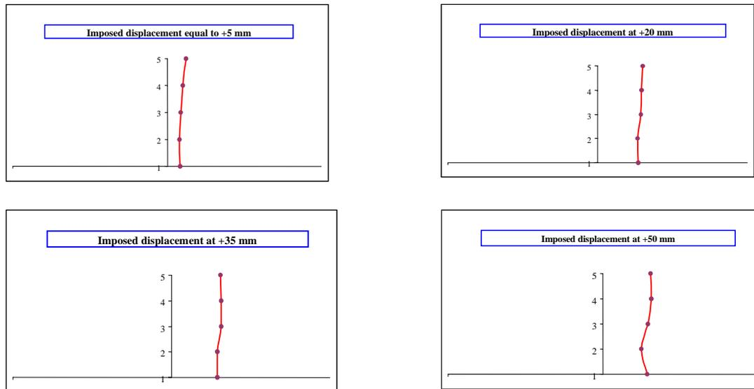
**Fig 11: Average distribution of the bending moment along the web profile**
