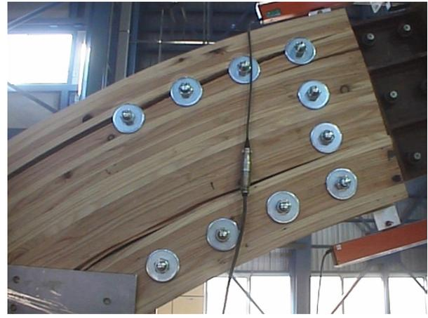
**Photo2 Splitting from bolt joint**
