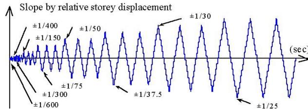
**Figure 3 Schedule of cyclic loading test**
