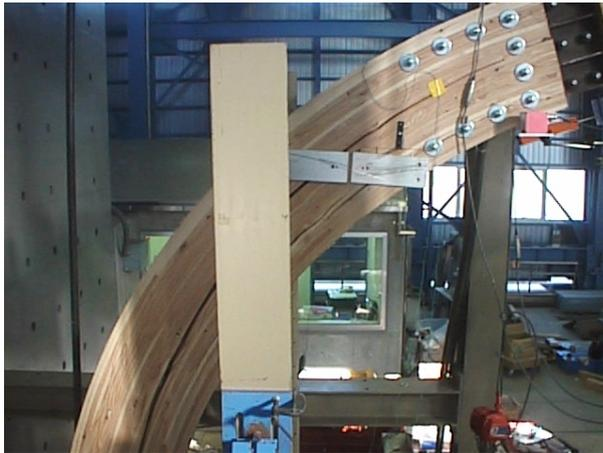
**Photo1 Shear failure of column**
