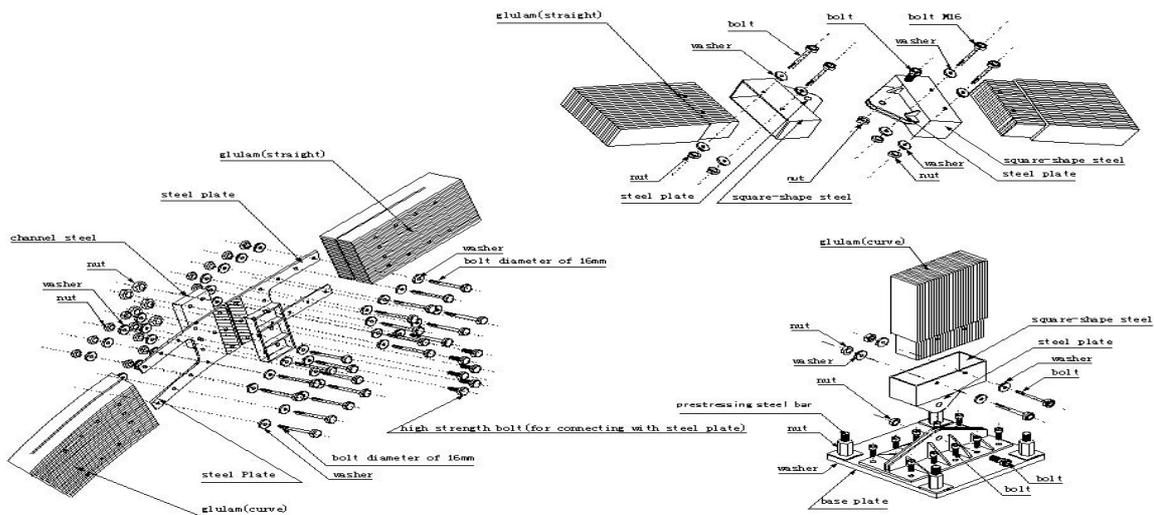
**Figure 2 Detail of joint**
