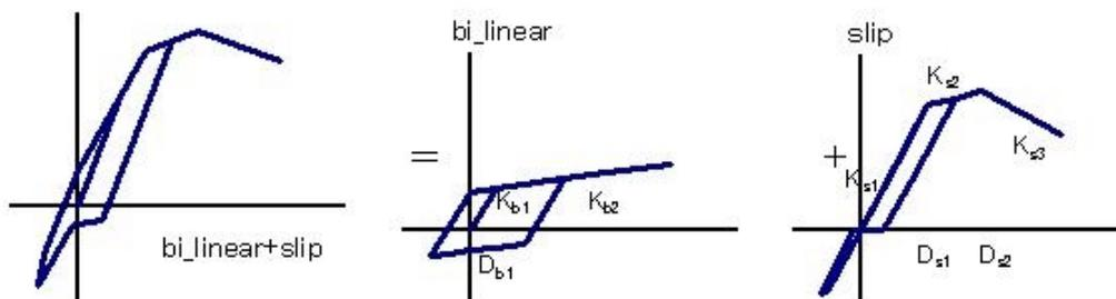
**Figure 7 Model of restoring force characteristic**
