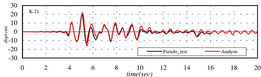
**Figure7 Comparison between pseudo-dynamic test and analysis**
