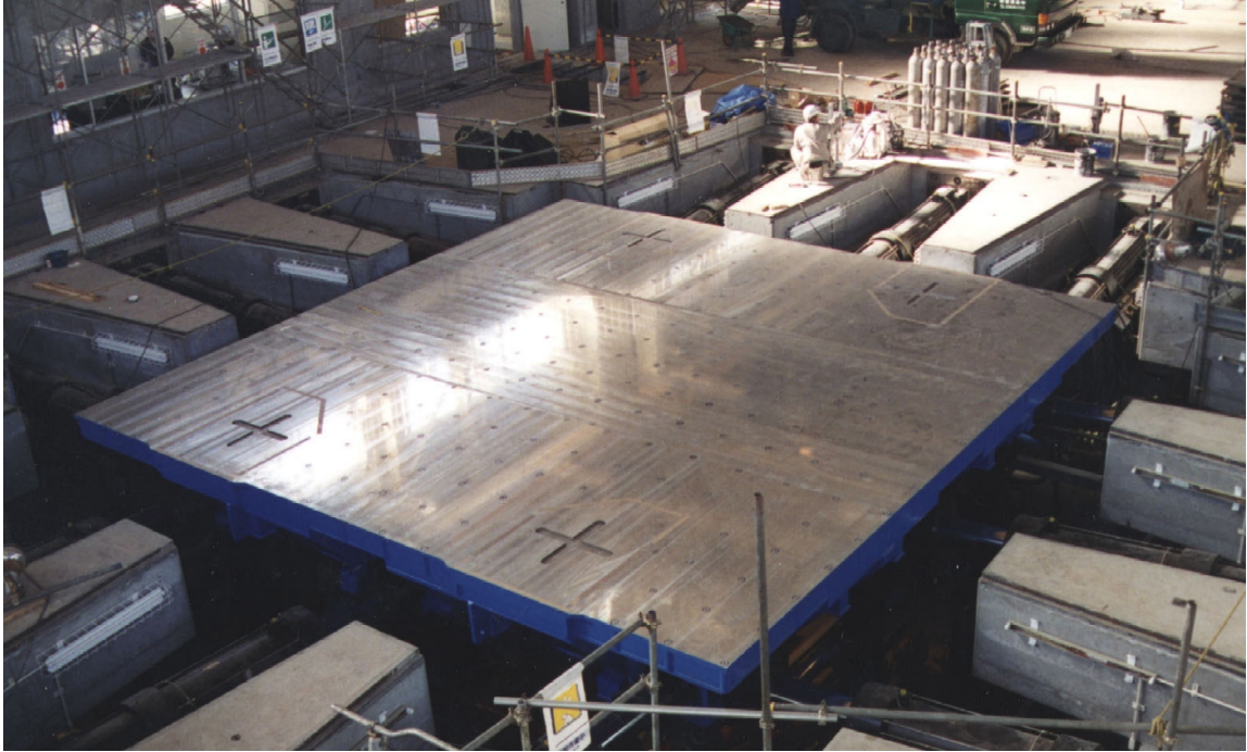
Figure 1 - PWRI-MOC 8x8 meter table under construction.
