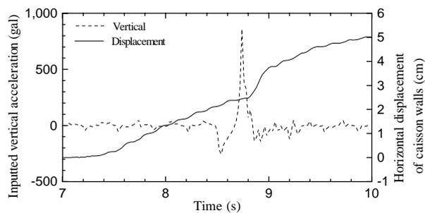
**Figure 6: Time histories of inputted vertical acceleration and displacement of caisson walls**
