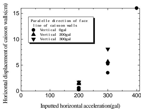
Figure 3: Horizontal displacement of caisson walls
