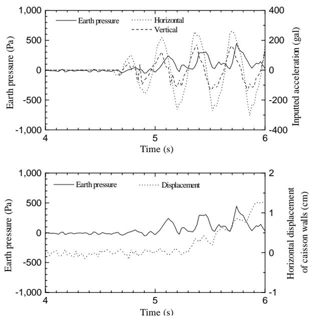
Figure 4: Time histories of earth pressure, inputted accelerations and displacement of caisson walls
