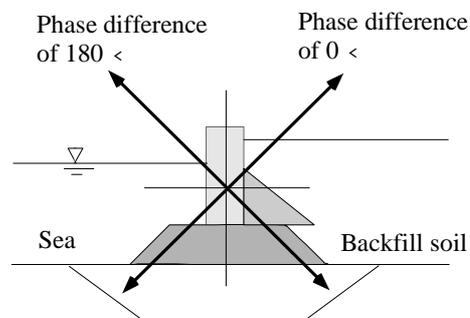
**Figure 7: Composite directions of inputted vertical and horizontal motions**
