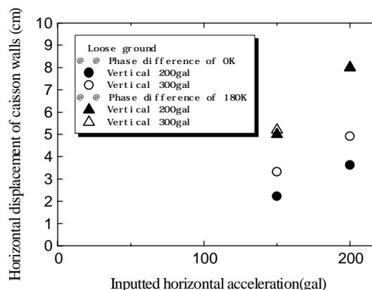
**Figure 10: Relationship between phase difference and displacement of the caisson walls at loose ground**
