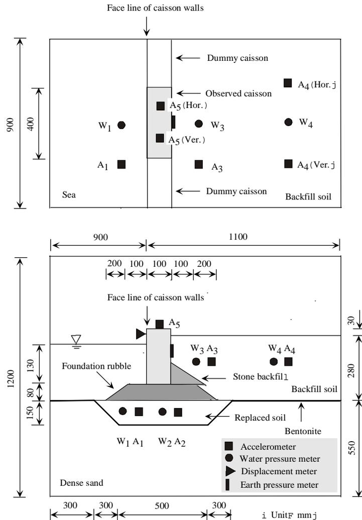
Figure 1: General view of test apparatus
