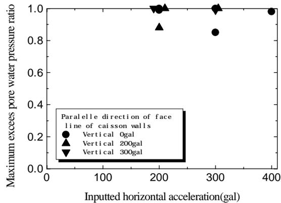
Figure 2: Maximum excess pore water pressure ratio of backfill soil
