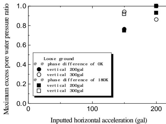
**Figure 9: Maximum excess pore water pressure ratio of the backfill soil**
