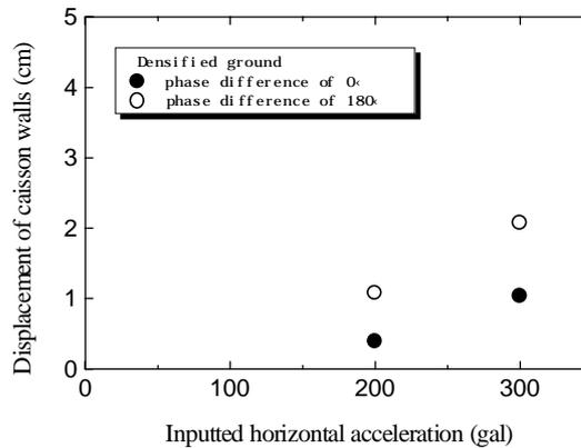
**Figure 8: Relationship between phase difference and displacement of caisson walls at densified ground**
