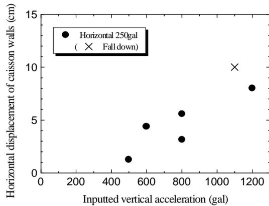
**Figure 5: Relationship between inputted vertical acceleration and displacement of caisson walls**
