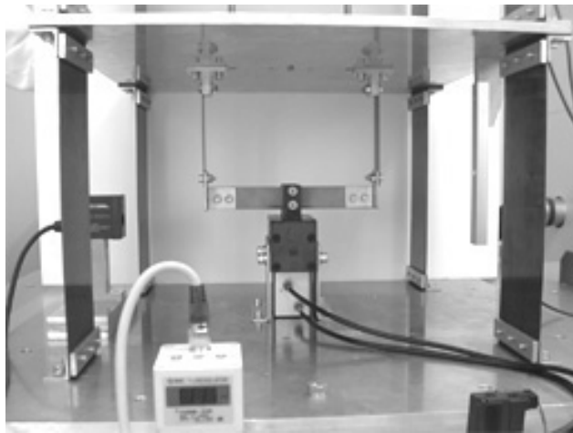
Figure 8: Photograph of air-cramp friction damper
