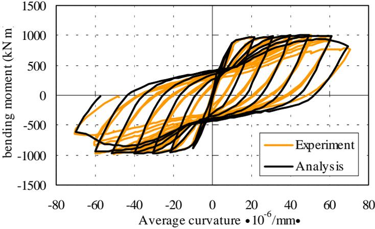
**Figure 10: Relationship between bending moment and average curvature**
