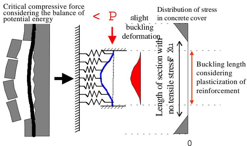
Figure 5: Method of predicting the spalling of concrete cover
