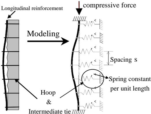
**Figure 3: Reinforcement buckling model**
