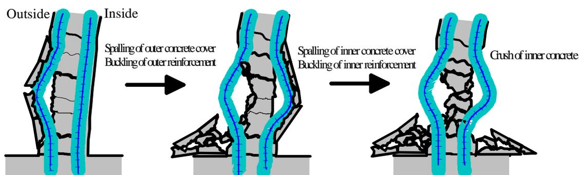
**Figure 1: Progress of failure at compressive flanges of a RC member with a hollow section**
