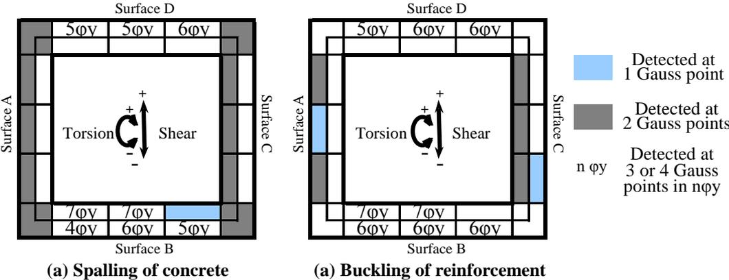
Figure 12: Prediction of timing of spalling and buckling at the bottom of the column
