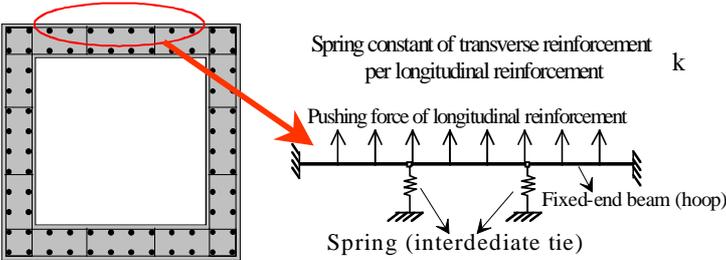
**Figure 2: Modeling of transverse reinforcement**
