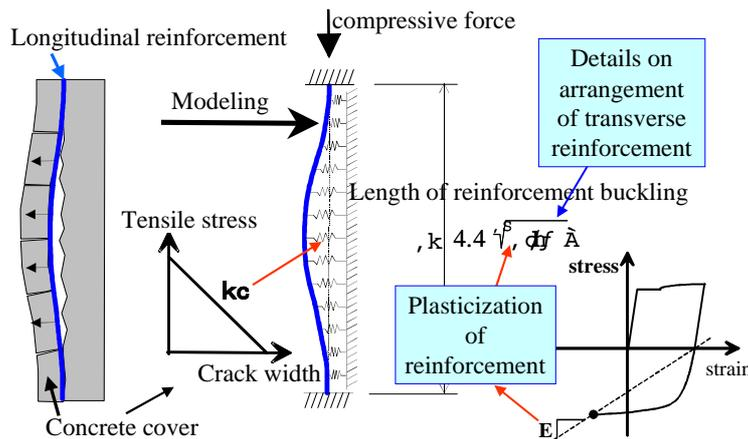
Figure 4: Concrete cover spalling model
