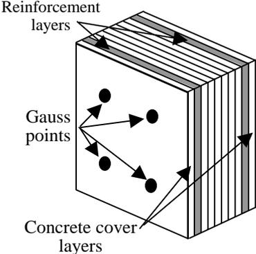
**Figure 8: Layers of shell element**
