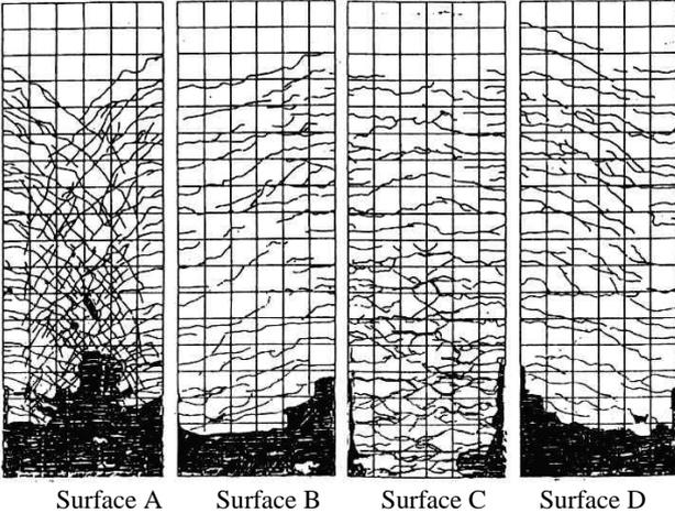
Figure 13: Cracking and spalling of the specimen after loading (10 cm per box)
