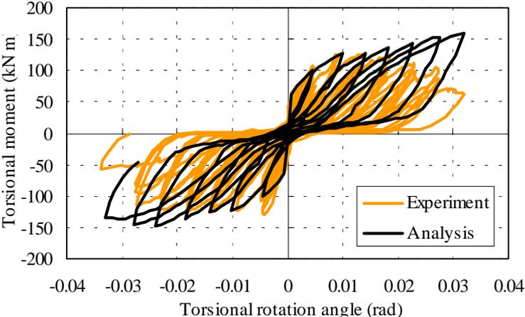
Figure 11: Relationship between torsional moment and torsional rotation angle
