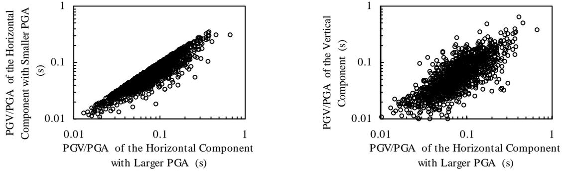
**Fig. 3 The Correlation of PGV/PGA Values of Three Components**
