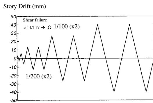
**Figure 11: Load Schedule for Static Test**
