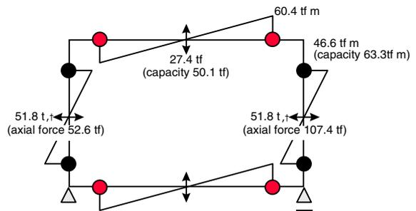
Figure 3: Failure Mechanism of the Specimen
