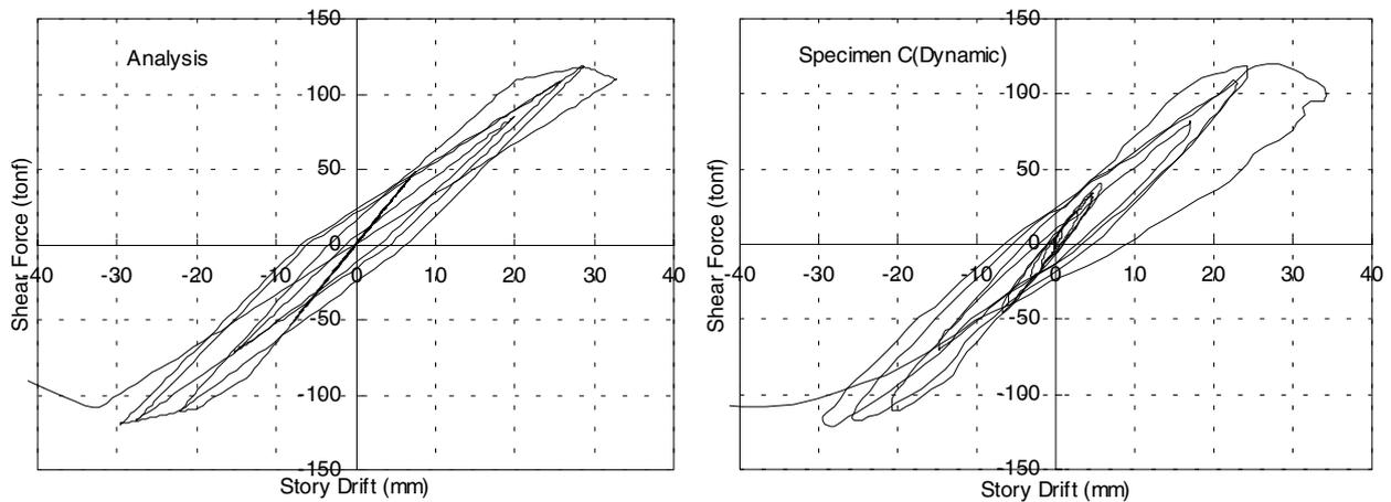
**Figure 15: Comparison of Load-Displacement Hysteresis**
