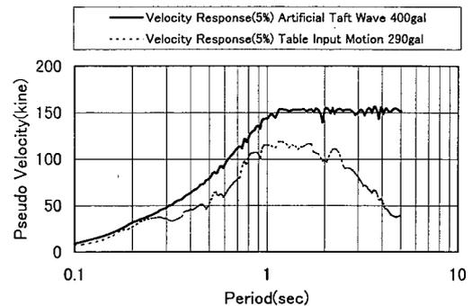
Figure 7: Velocity Response Spectrum
