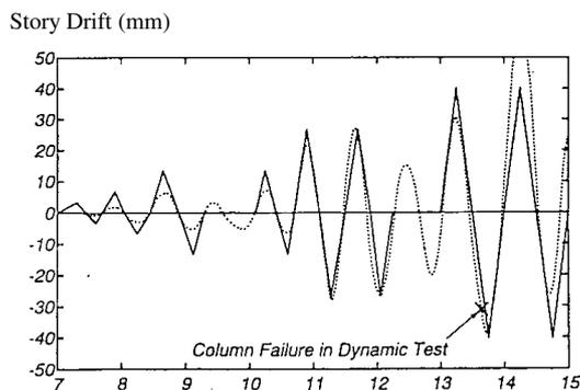
**Figure 10: Inter Story Drift (dynamic test)**
