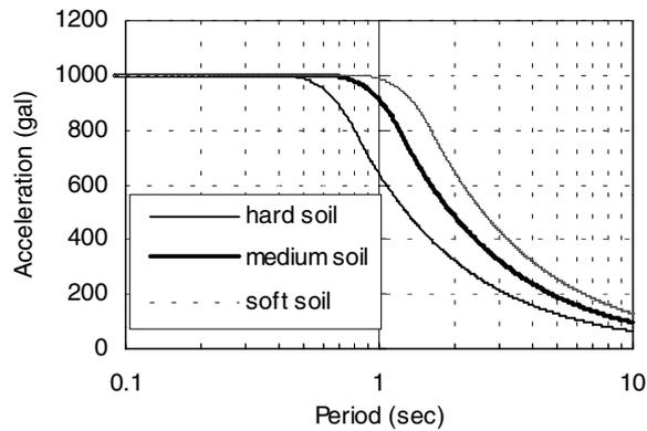
Figure 5: Acceleration Response Spectrum Corresponding to the Building Regulation in Japan
