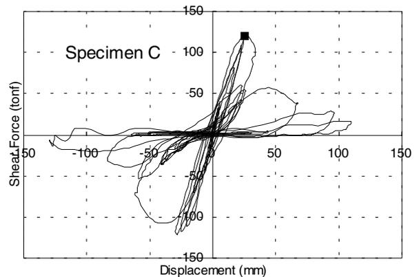
**Figure 8: Shear Force-Displacement Hysteresis (■ indicates shear failure of columns)**
