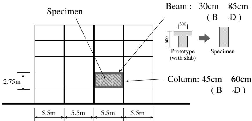
Figure 1: Original RC Structure and Modified Dimensions for the Test Specimen
