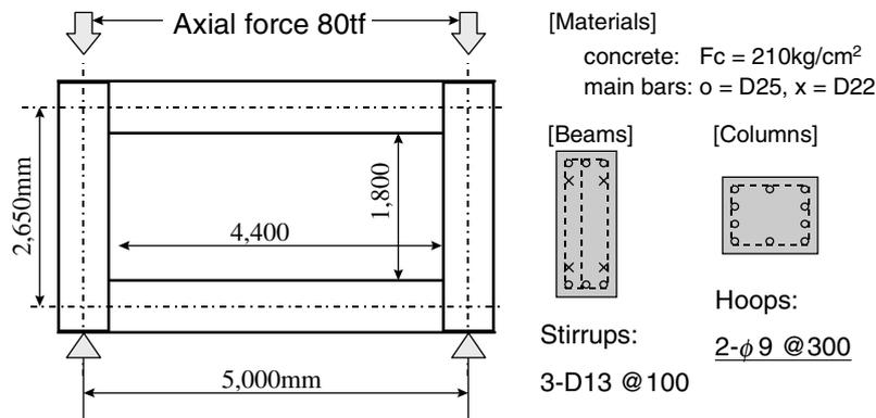
Figure 2: Dimensions of RC Specimen and Arrangement of Steel Bars
