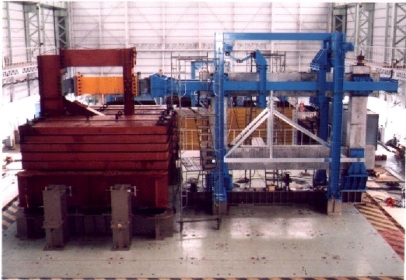
**Photo 1: Experimental Facility on Shaking Table (in Science and Technology Agency)**
