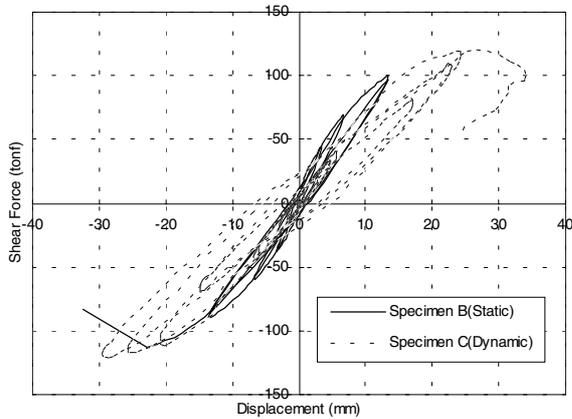
Figure 12: Comparison of Dynamic and Static Test
