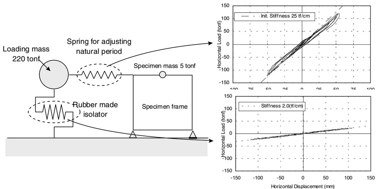
Figure 14: Analytical Model for Equipment
