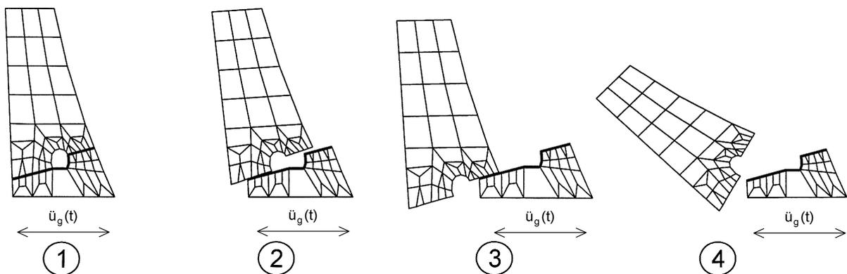
**Fig. 7 Failure mode of the dam obtained from dynamic analysis for earthquake excitation with peak ground acceleration of 2 g (sliding failure)**
