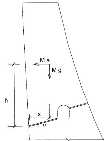
Fig. 2 Critical pseudostatic accelerations for sliding and overturning of detached upper portion of dam
