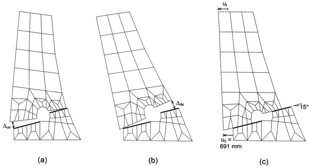
**Fig. 4** (a) and (b) show the rocking of the detached upper portion of the dam during earthquake shaking, and (c) shows the final configuration with permanent sliding displacement after an earthquake with a peak ground acceleration of 0.5 g (coefficient of friction in crack: 0.7)
