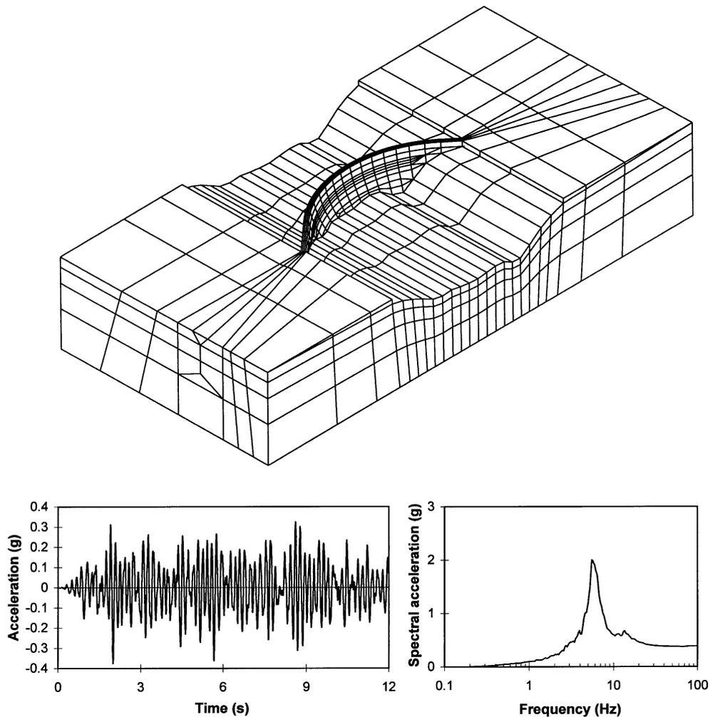
**Fig. 3 Three-dimensional dam-foundation model (top) and time history of radial acceleration at base of upper gallery with corresponding floor response spectrum for PGA of 0.1 g (bottom)**
