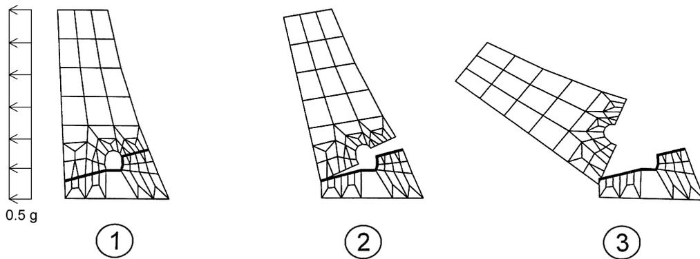
**Fig. 6 Failure mode of the dam obtained from pseudostatic analysis (rocking failure)**
