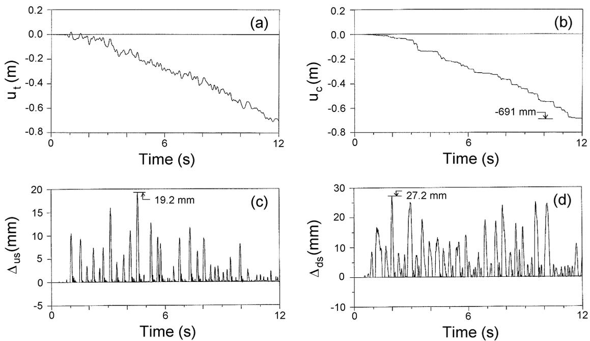
**Fig. 5** Time histories of (a) radial displacement of dam crest, (b) sliding movement towards upstream along crack surface, (c) crack opening at upstream dam face and (d) crack opening at downstream dam face for earthquake excitation with peak ground acceleration of 0.5 g (coefficient of friction: 0.7; crack inclination: 15°)
