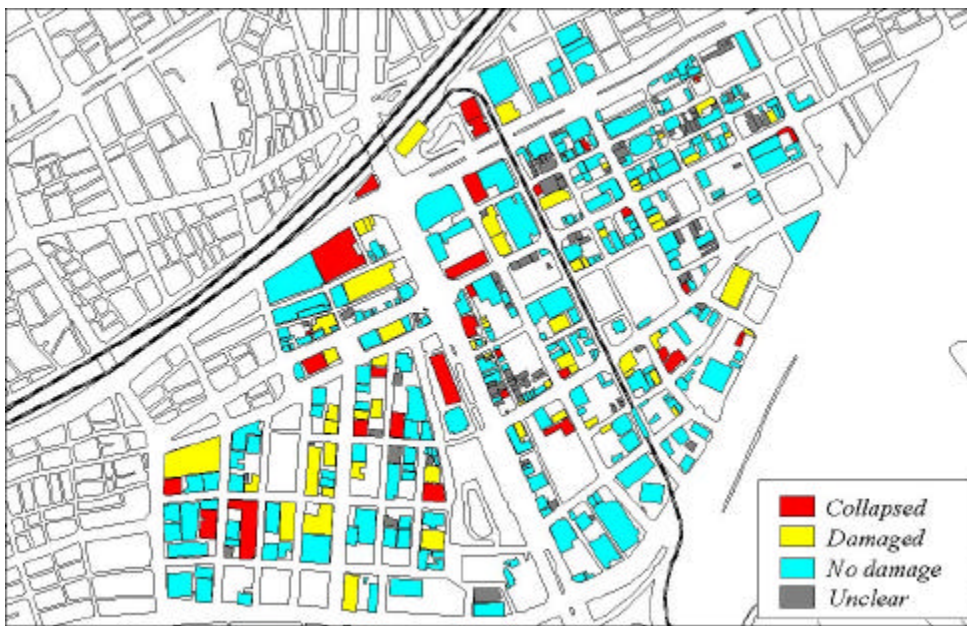
Figure 6: Distribution of building damage in Area 2 interpreted from the aerial HDTV images
