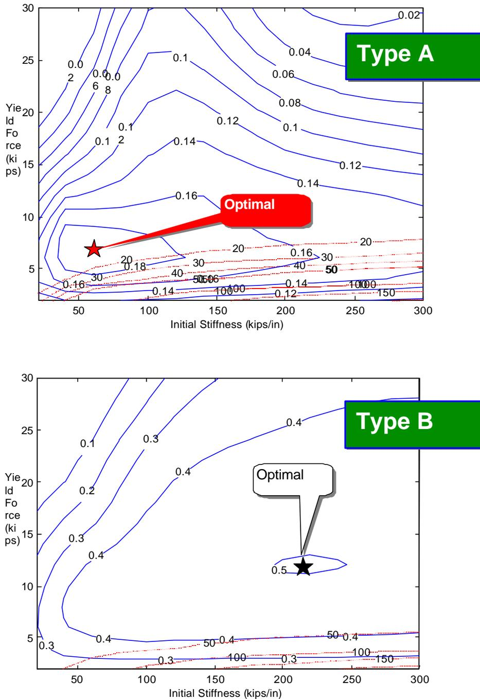
**Fig. 9: Design Results for Type A and Type B PED Concepts**
