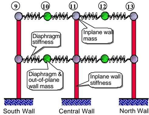
**Fig. 4: Plane Frame Model of Low Rise URM Building**
