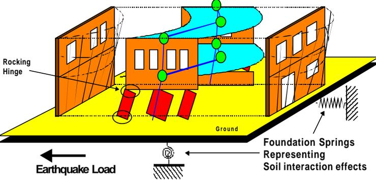
Fig. 2: Conceptual Model of Low Rise URM Building
