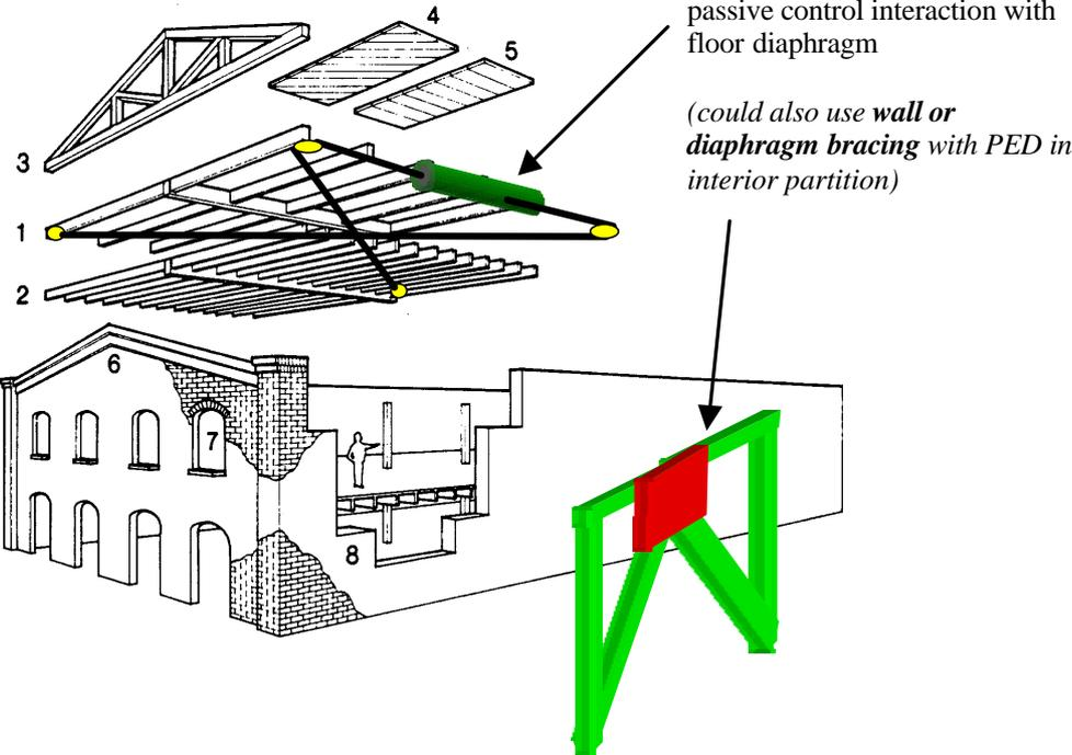
Fig. 3: Applications of PED's Within Low Rise URM Buildings
