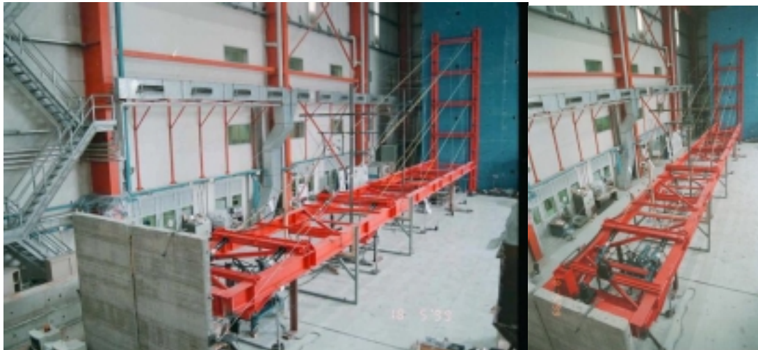
Figure 4 – The large scale test on a suspended bridge in progress at the Joint Research Center in Ispra
