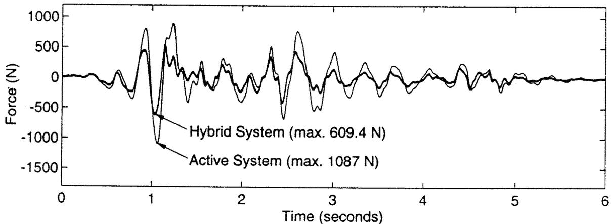
Figure 4: Comparison of required active control forces
