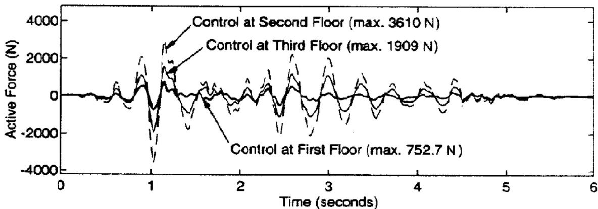
Figure 7: Required active control force for scaled el centro earthquake
