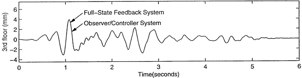
Figure 6: Comparison of closed-loop displacement responses
