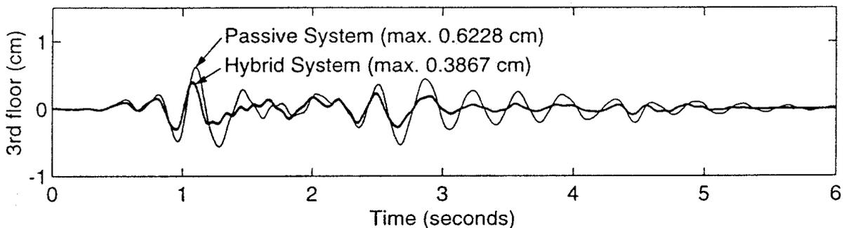
Figure 5: Comparison of displacement responses at third floor
