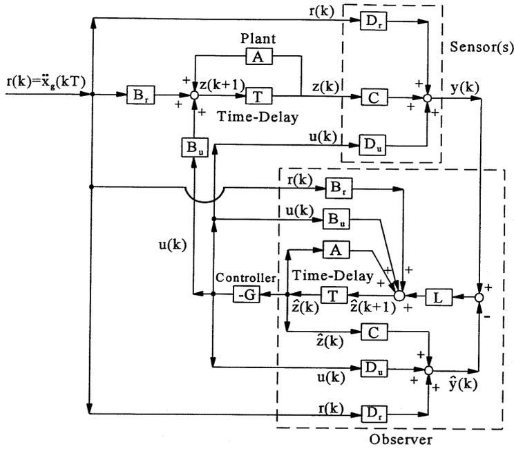
Figure 2: Simulation diagram of observer-controller system
