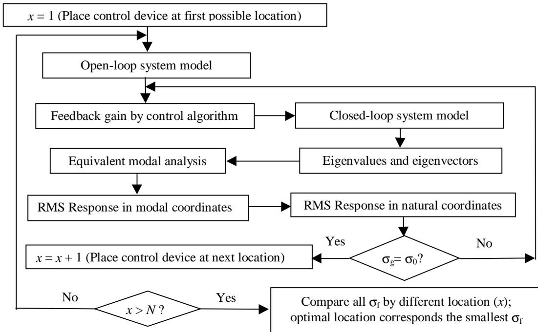
Figure 3: Flow of solution procedure for optimal placement problem
