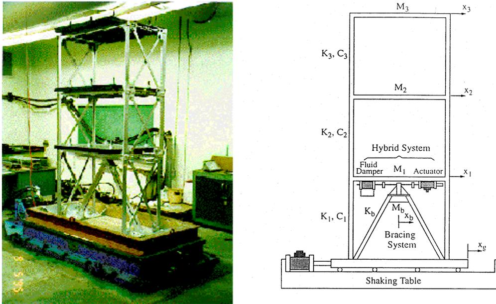
**Figure 1: Structural model and hybrid control system for shaking table test**
