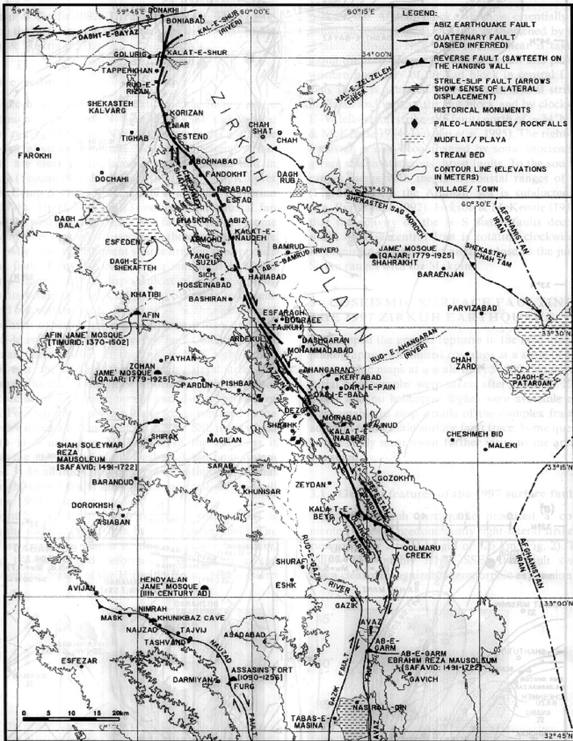
Figure 3. The causative fault of the Ardekul destructive earthquake (After Berberian et al., 1999)
