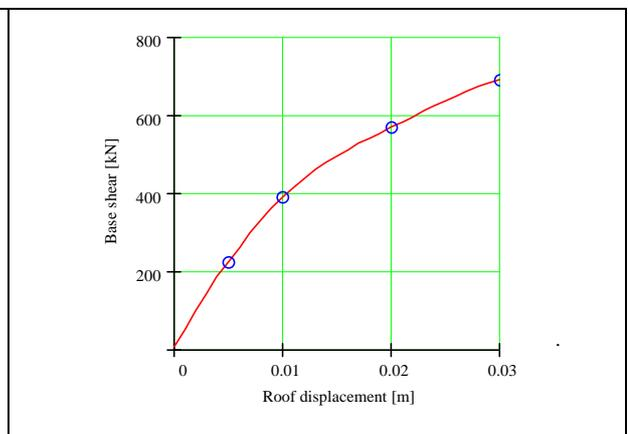
Figure 45. building B - capacity curve
