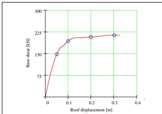
Figure 44. building A - capacity curve
